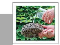
Figure 1: Image of water seepage through porous concrete.<sup>53</sup>
